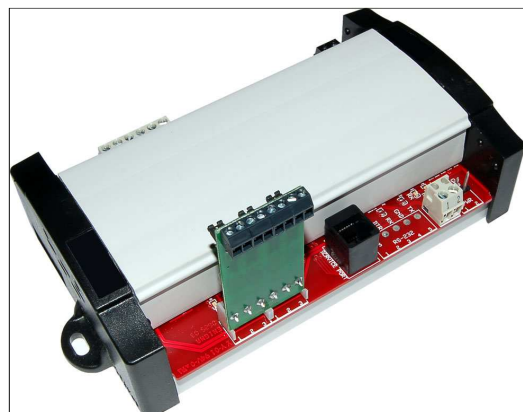
ETHP4 mounted on DDC controller
